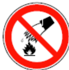
Extinguishing with water prohibited
