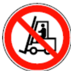
Prohibited for floor vehicles
